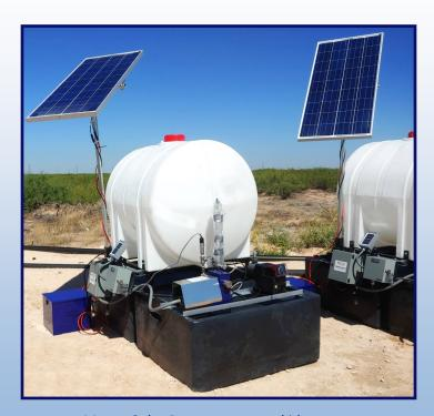
Megas Solar Pump set up on skid
